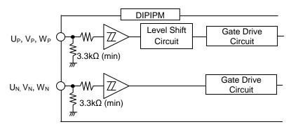
Fig.3-4 Internal structure of control input terminals
