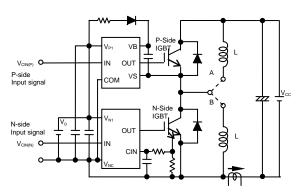
Short A for N-side IGBT, and short B for P-side IGBT evaluation Fig.2-3 Evaluation circuit (inductive load)
