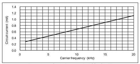
Fig.4-4 I<sub>DB</sub> vs. Carrier frequency for PSS10SA2FT
