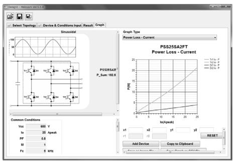
Fig.3-22 Loss simulator screen image
