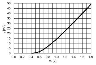
Fig.4-9 V<sub>F</sub>-I<sub>F</sub> curve for bootstrap Diode (The right figure is enlarged view)
