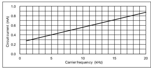
Fig.4-3 I<sub>DB</sub> vs. Carrier frequency for PSS05SA2FT
