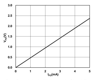
Fig.3-7 Fo terminal typical V-I characteristics (V<sub>D</sub>=15V, T<sub>i</sub>=25°C)
