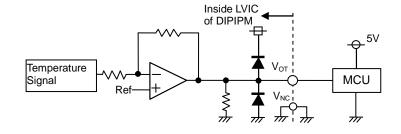
Fig.2-10 Inner circuit of V<sub>OT</sub> terminal
