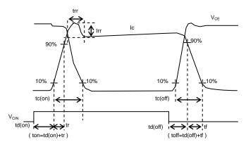
Fig.2-2 Switching time definition
