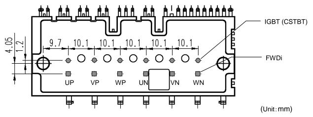
Fig.2-19 Power chip position
