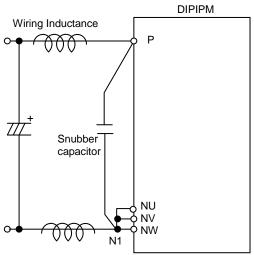
Fig.3-8 Recommended snubber circuit position
