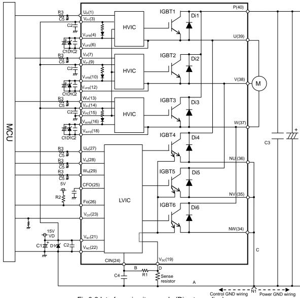
Fig.3-2 Interface circuit example (Direct coupling)
