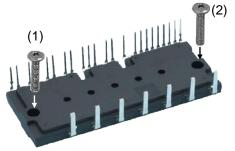
Fig.2-21 Recommended screw fastening order
