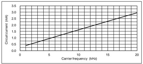
Fig.4-8 I<sub>DB</sub> vs. Carrier frequency for PSS50SA2FT
