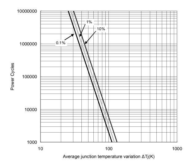
Fig.3-19 Power cycle curve
