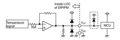
Fig.2-12 V<sub>OT</sub> output circuit in the case of using with low voltage controller
