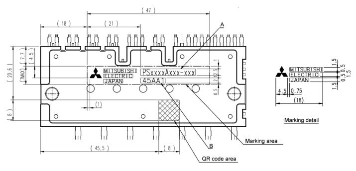
QR code is registered trademark of DENSO WAVE INCORPORATED in JAPAN and other countries.  $\mbox{Fig.2-20 Laser marking view}$
