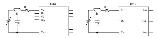
Fig.3-25 Surge test circuit example(V<sub>N1</sub> terminal)
