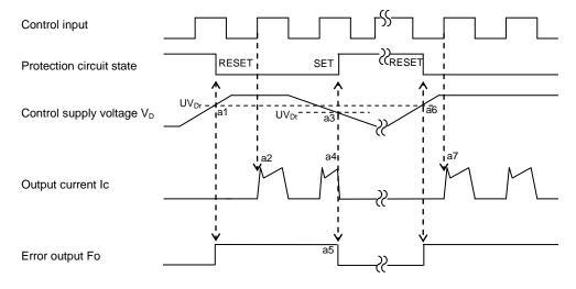
Fig.2-8 Timing chart of N-side UV protection
