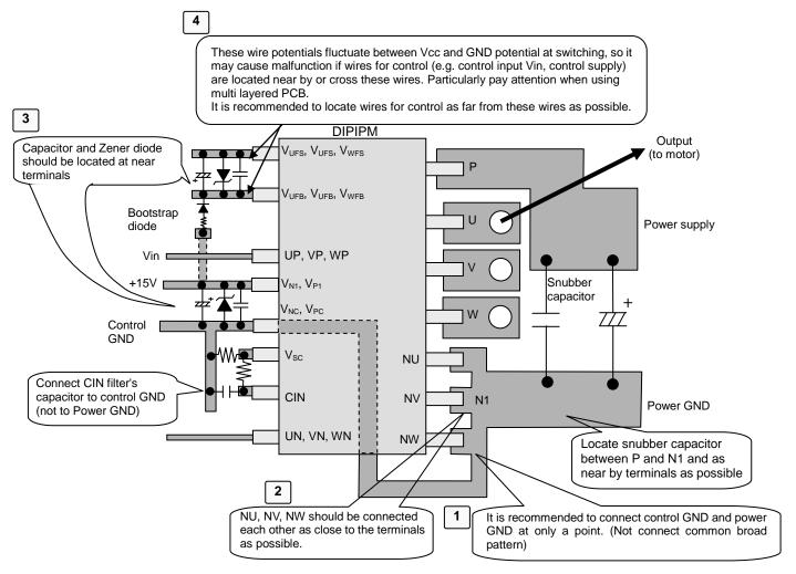
Fig.3-10 Precaution for wiring on PCB
