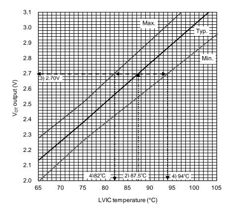
Fig.2-17 V<sub>OT</sub> output vs. LVIC temperature (Enlarged graph of Fig.2-14)
