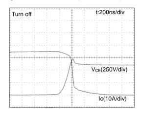
Conditions:  $V_{CC}$ =600V,  $V_D$ = $V_{DB}$ =15V, Tj=125°C, Ic=35A, Inductive load half-bridge circuit
