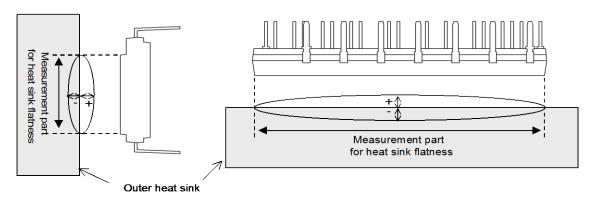
Fig.2-22 Measurement point of heat sink flatness
