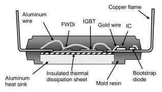
Fig.1-2 Internal cross-section structure
