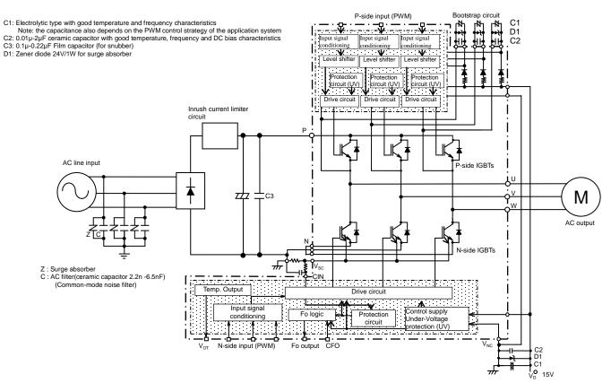
Fig.3-1 Application System block diagram
