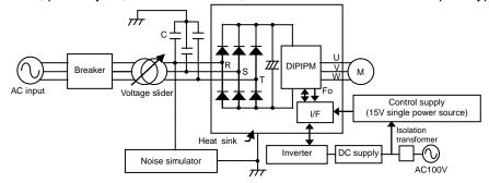
Fig.3-23 Noise withstand capability evaluation circuit
