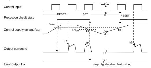
Fig.2-9 Timing Chart of P-side UV protection
