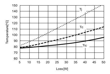
Fig.2-15 IGBT loss vs. Tj, Tc, Tic(Typical) (Ta=80°C)
