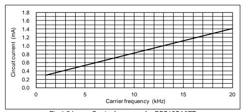
Fig.4-5 I<sub>DB</sub> vs. Carrier frequency for PSS15SA2FT
