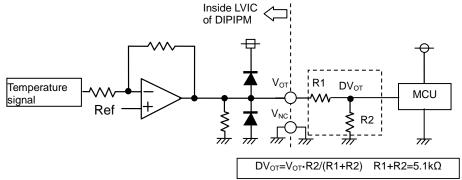
Fig.2-13 V<sub>OT</sub> output circuit in the case with high protection level
