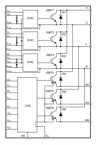
Fig.1-3 Internal circuit schematic
