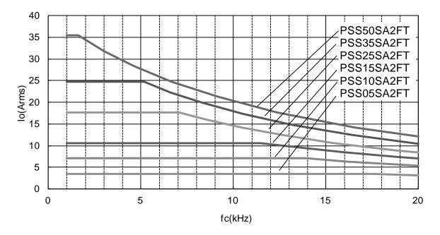
Fig.3-21 Effective current-carrier frequency characteristic
