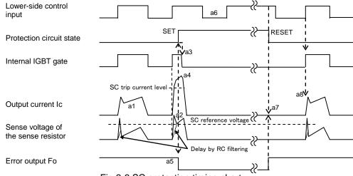
Fig.2-6 SC protection timing chart
