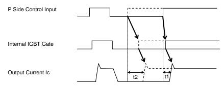
Real line: off pulse width>PWIN(off); turn on time t1 Broken line: off pulse width<PWIN(off); turn on time t2 (t1:Normal switching time)
