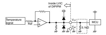
Fig.2-11 V<sub>OT</sub> output circuit in the case of detecting low temperature
