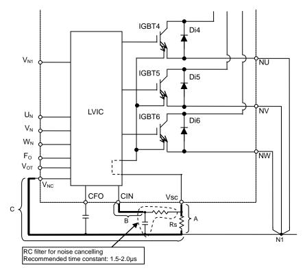
Fig.3-9 External protection circuit
