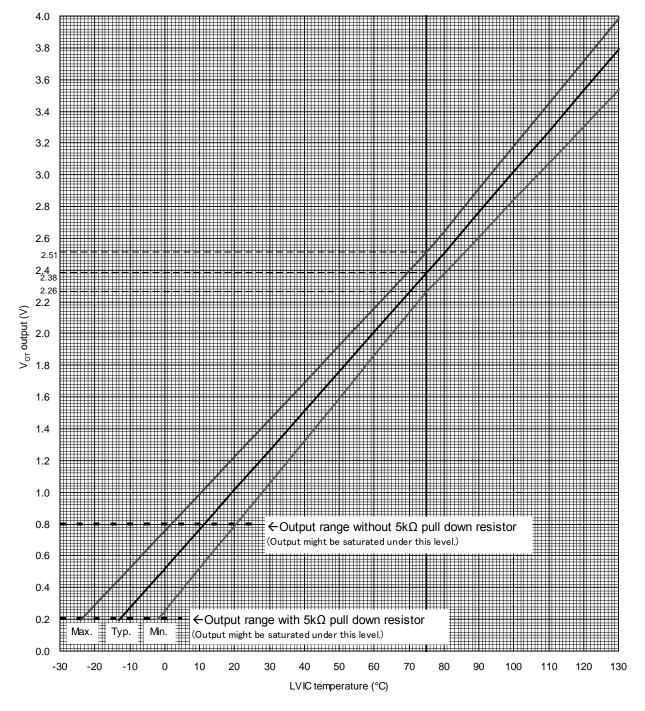
Fig.2-14  $V_{\text{OT}}$  output vs. LVIC temperature
