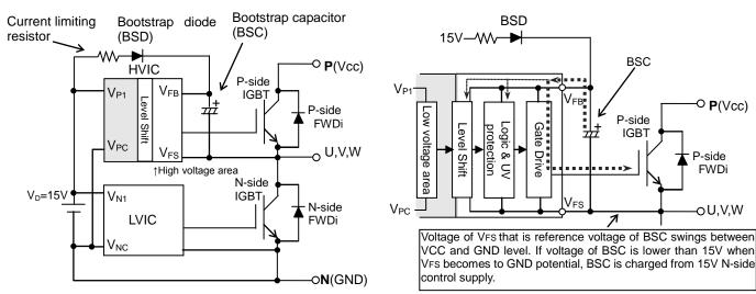
Fig.4-1 Bootstrap Circuit Diagram
