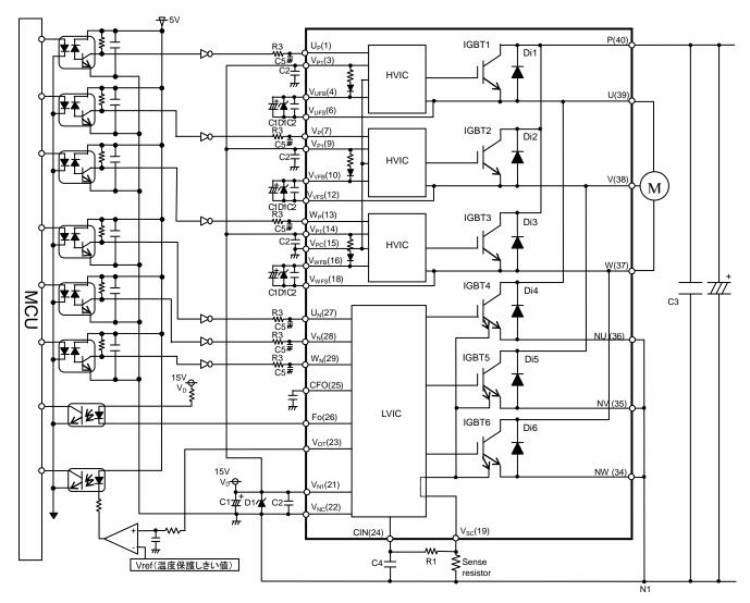
Fig.3-3 Interface circuit example with opto-coupler
