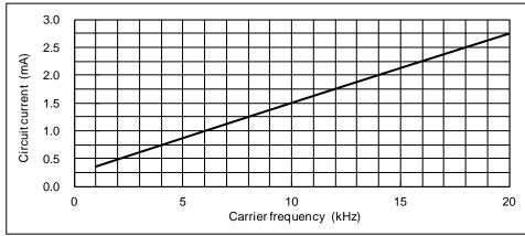
Fig.4-7 I<sub>DB</sub> vs. Carrier frequency for PSS35SA2FT
