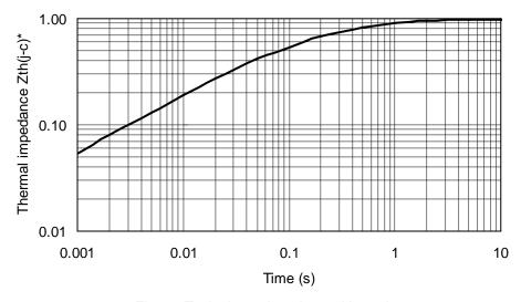
Fig.2-1 Typical transient thermal impedance
