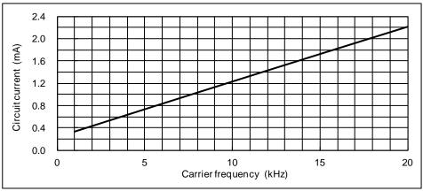
Fig.4-6 I<sub>DB</sub> vs. Carrier frequency for PSS25SA2FT
